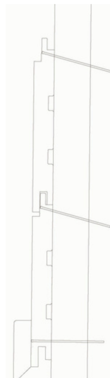
Example of concealed fixing
